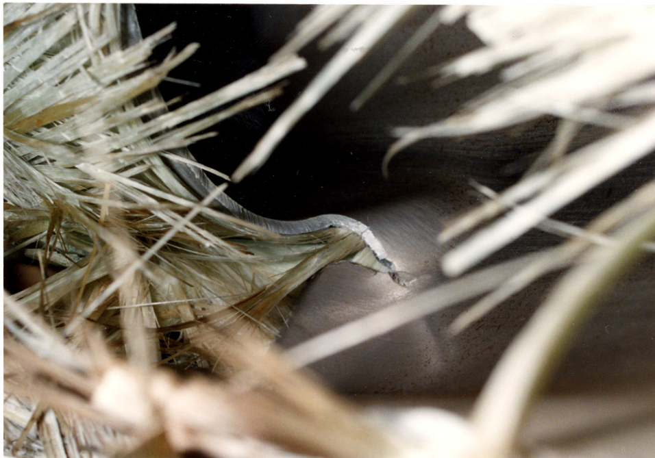
44. Close-up view of a fracture line in the aluminum tank along the bottom left side
